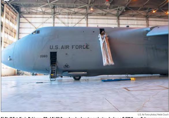
5) Staff Sgt. Kevin Robinson. 22nd Airlift Squadron loadmaster evaluator, deploys a C-5M Super Galaxy emergency escape slide Sept. 6 at Travis Air Force Base. Robinson wore a GoPro camera to record the process which will be used to develop a virtual reality training program on aircraft procedures.
